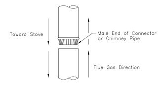
FIGURE 2.3 (A) Connecting Sections
